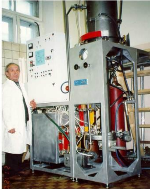
Gravity-type furnace for production of microspheres
